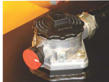
Integrated oil filter with Breather
