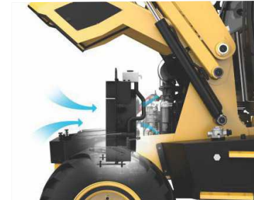
Single layer Radiator/ Cooler: Easy to clean
